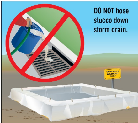
Large concrete washout fabricated from straw bales or filter socks, plastic sheeting, and wooden stakes. Note how sheeting extends well over sidewalls, and is tucked under bales.
